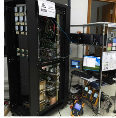
Fig. 11. Experimental setup of the 110 V-5 kV-A TCLC-HAPF experimental prototype.
